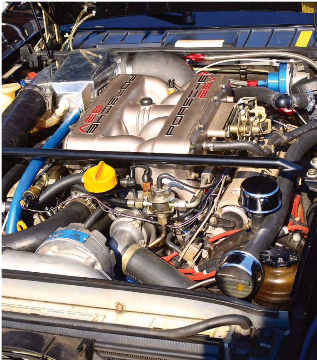
Below: Not your normal 928 engine bay. Notice the Vortex supercharger at the engine's front and the modified air intake toward its rear.
