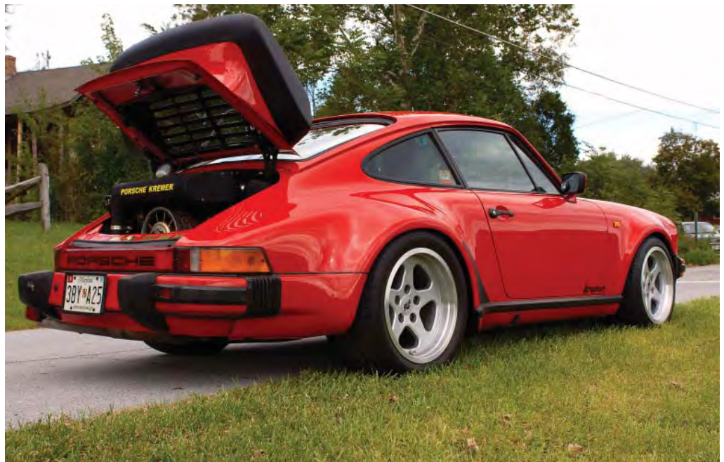
Top: Kremer's massive intercooler assists in producing much of the additional 90 hp. Bottom: Stylish 17inch Ruf Speedline wheels were added after importation to the US.
