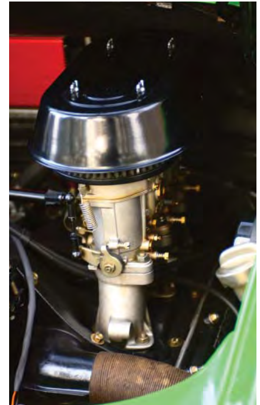
The engine features a high-lift cam to extract the best range of power from its PMO 46 MM carburetors. Compression is 10.5:1 using Mahle high-domed, Nikasil-coated pistons. The 3.2 flat-6 produces nearly 300 hp at the fly.
